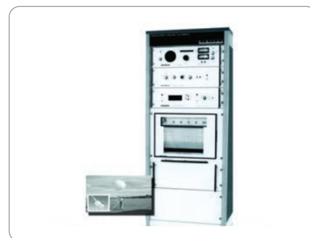
4 Radiosonde Ground Equipment
